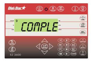
9. After the final ingredient has been loaded RECIPE COMPLETE TOTAL LOADED XXX KG will be displayed.
