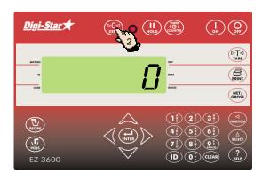
2. Press and hold (PO) for 3 seconds to zero balance the weighing indicator.
