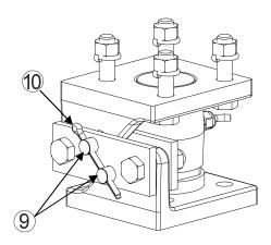
For mobile applications, an anti-rotation device may be required to prevent load cell cable damage. Below are two possible methods:
