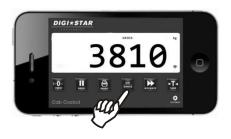
5 Press to display the total amount loaded. In this example: 1250 kg + 2560 kg = 3810 kg. "Gross" (Gross mode) is displayed in the header.
